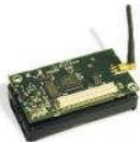
**b. Sensor Board:** MDA100 sensor and data acquisition board includes a precision thermistor, a light sensor/photocell and provides a general prototyping area.
