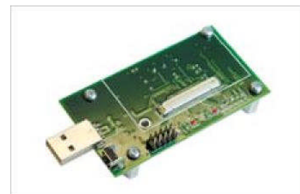
MIB520CA Mote Interface Board
